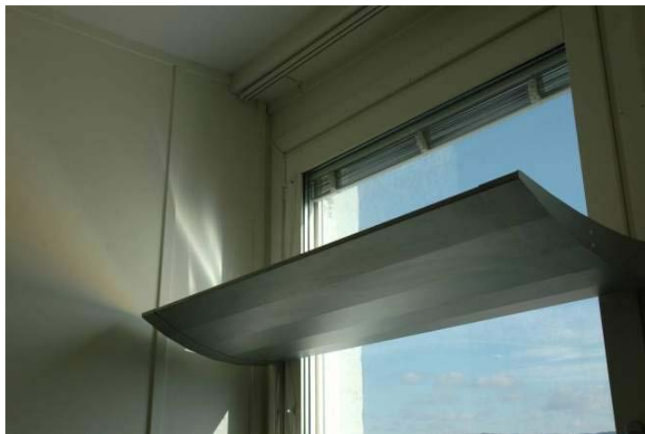
Figure 5-28. A prototype of the Daylight Luminaire. Upward reflected sunlight as well as electric light can be seen on the wall to the left of the luminaire.
