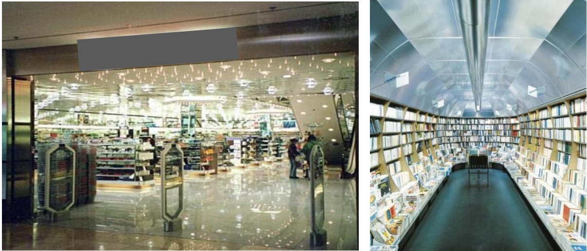
Figure 8-3. Comparison of shop lighting: left the light points are in the focus, right the ware (Bartenbach 2009).
